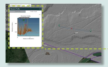
Measure 3D feature heights easily with the ability to draw lines over multiple surfaces to visualize canopy and building height comparison profile graphs.
